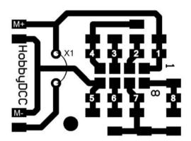
**M+ / M- and 1 / 5:** Motor red and black (blue) output. Polarity may be changable by inserting X1.
