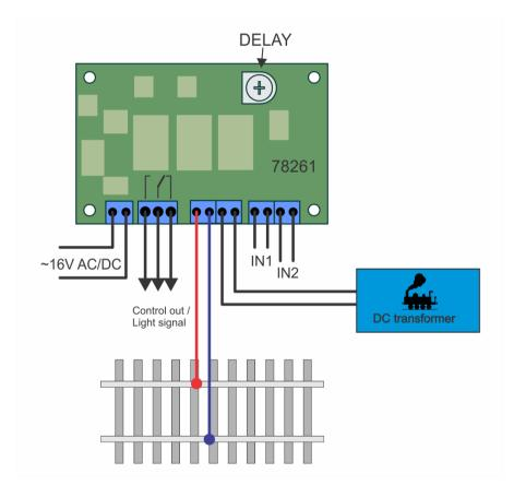
Figure 2: Connection of the control inputs at the two terminals
